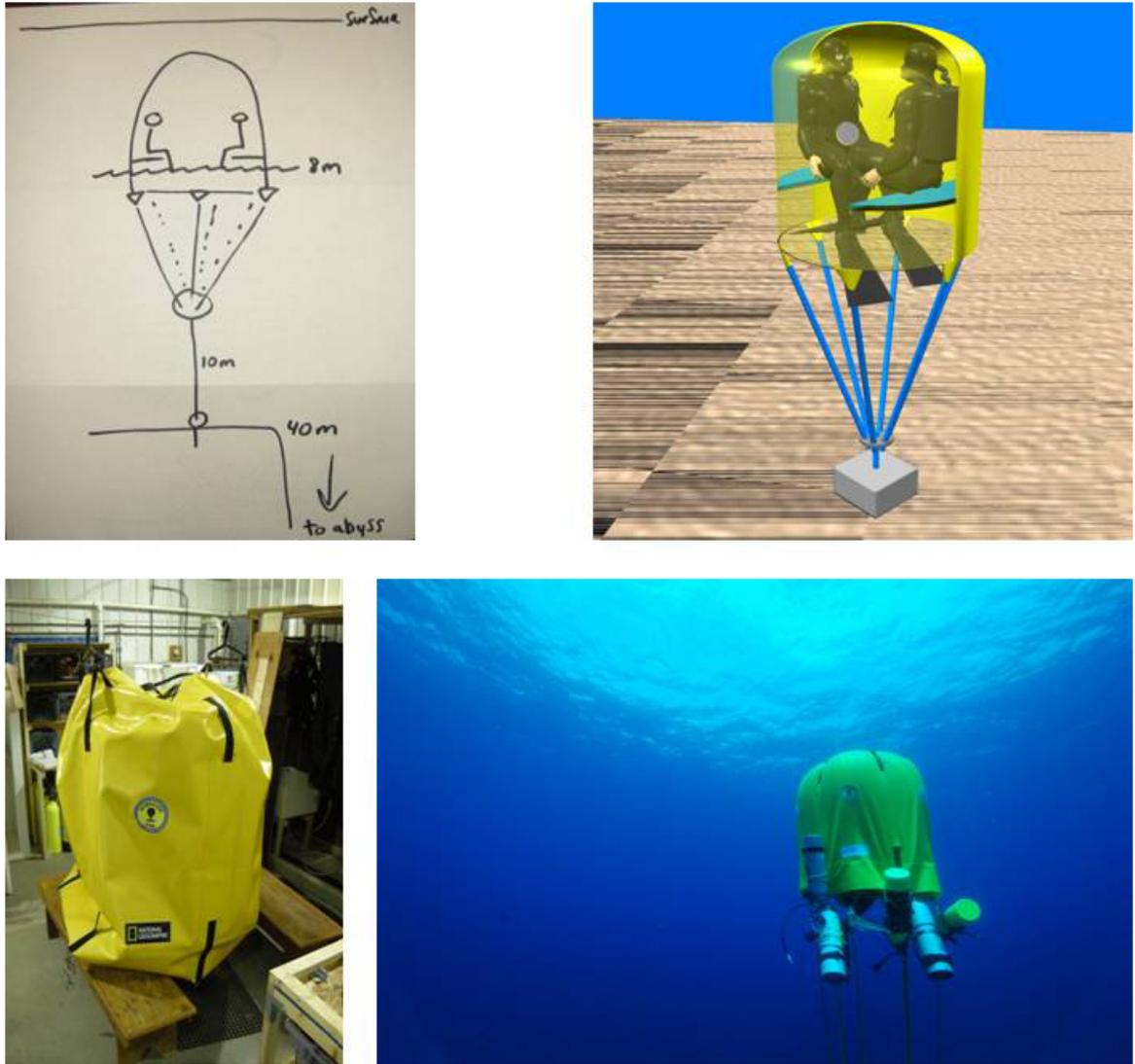
Figure 1: (top left) Concept sketch of habitat deployed along vertical wall. (top right) Rendered solid model of Gen 1 system, courtesy Anthony Appleyard. (bottom left) Prototype Gen 1 system prepped for deployment at University of Rhode Island. (bottom right) Gen 1 system deployed in Bahamas at 20 fsw, photo courtesy of National Geographic Society/Waite Grants Program.
